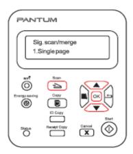
**Step 2:** Press "▲" or "▼" button to select and enter "Merge Scan" mode.
