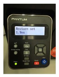
For M6600 Series printer, Here is the way to recover factory default setting in case customer forgets the password:
